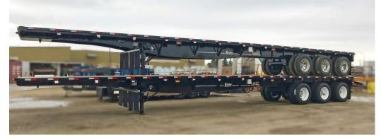
Suspension: Sliding Hendrickson AAT23K INTRAAX Air Ride with 3-23,000lb axles, 60"-60" Spread - Kingpin to C/L Middle Axle: Front Position 452", Kingpin to C/L Rear Position 519", 17" Ride Height, 77 1/2" Track Width: HXL5 Wheel Seals Federal Moaul
