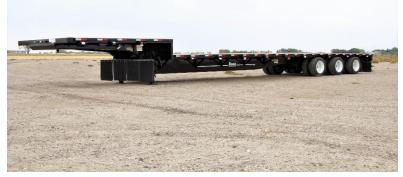
**Coating:** All Components Steel Shot Blasted, PPG Zinc Rich Epoxy Primer Inside and Out, Top Coat PPG Urethane, All Painted Parts Baked in Heat Ovens
